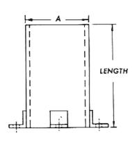
Pipe Sleeves are cut from standard weight pipe (Schedule 10, Schedule 40) and are furnished with welded lugs.
